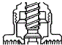
螺纹旋进阀盖 Threaded-in Bonnet
